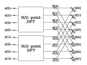
Fig 3 Data Flow Diagram for N=8: A Decimation-In-Time Radix-2 FFT
