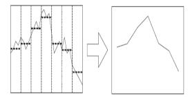
Fig. 2 Time Series Dimensionality Reduction by PAA the Horizontal Dotted Lines Show the Mean of Each Segment.
