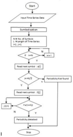
Fig. 6 Flowchart for periodicity detection [11]
